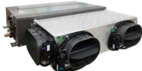
Complete of oval connections made of PVC, with insulation external and elastic sheath for the joint to the ventilating unit. The use of PVC ensures the best quality of air combined with the extreme lightness and long lasting. Equipped with practical kit of thermoregulation complete with motorized dampers already installed, the power module evolved from 2 to 6 zones, 12V power supply, already wired.
